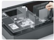
The innovative design is composed of a ventilation box, a honeycomb table and rearrangeable magnetic supporting pieces. The SmartBOX  $^{\mbox{\scriptsize TM}}$ provides great cutting quality and remarkably enhance air extraction.
